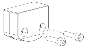
For the tool changers TC240, TC480 and TC720, equipped with safety signal module P7501xxx, the tool in stand sensor P8369 shall be mounted on tool stand hanger and used together with I1171 mounted on the tool plate.
