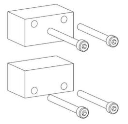
Spacers for mounting of passive tool in stand sensor P8369 on the tool hanger and the tool in stand sensor I1171 on the tool plate.
