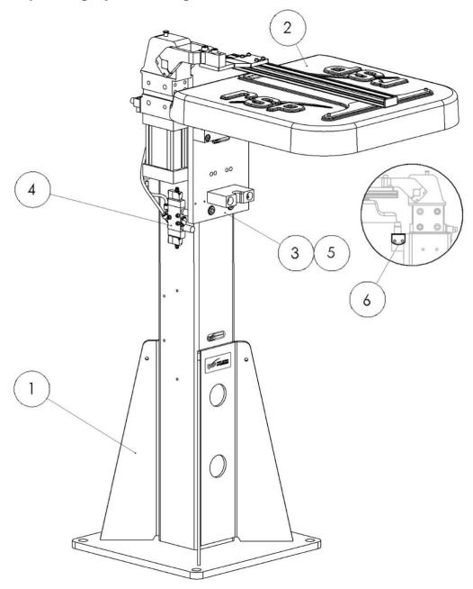
Tool parking system single P8365 and P8385 shall be used together with the tool changers TC240, TC480, TC720 and corresponding tool attachments. P8365 should be used together with safety signal modules P7501-xxx. P8385 can be used together with tool in stand sensor assembly, P8364, and tool present sensor, P8312.
