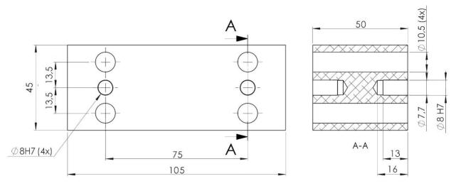
The spacer P0186-049 shall be mounted between the tool attachment and tool plate.
