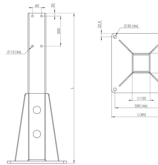
The tool stand column P8380 gives together with the tool hanger P8302 and tool plate P8303A a robust tool parking system for easy tool changing. The tool stand column comes in different heights and is prepared for mounting of a single or double hanger, dust cover, connection modules and valve units.
