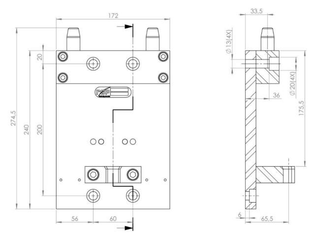
The tool hanger P8302, mounted on the tool stand column P8380, gives together with tool plate P8303A a robust tool parking system for easy tool changing. To be mounted using mounting kit for tool hanger, P8370.
