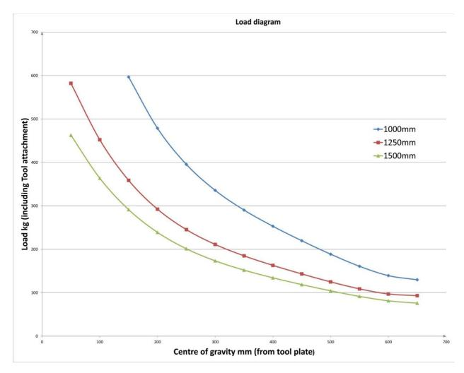
The diagram shows the load corresponding to a maximum displacement of 0.5 mm of the tool (including tool attachment) at its point of gravity.
