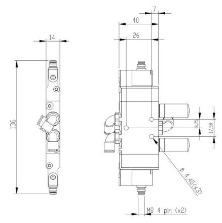
A bi-stable 5/2-valve to be mounted on the tool stand column P8380 and used together with P8327, P8377 or P8379 (dust covers with pneumatic tilting clamps).
