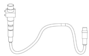
To be mounted on the tool hanger, a 0.8 meter cable is included. Transmits a double channel signal to detect presence of tool in the tool parking system.
