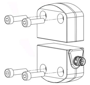
For the tool changers TC240, TC480 and TC720 without safety signal module and the tool changer TC500. The active tool in stand sensor P8382 can be mounted on tool stand hanger and the passive part mounted on the tool plate.
