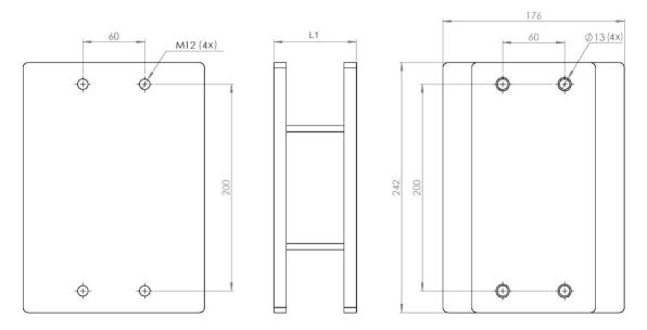
The tool hanger extension P8371 shall be mounted between the tool stand column, P8380, and the tool hanger, P8302 in combination with dust cover with pneumatic tilting clamp large, P8327/P8377. The tool hanger extension P8381 shall be used in combination with dust cover with pneumatic tilting clamp small, P8379. When required an extra-long aluminium profile for the dust cover is included.
