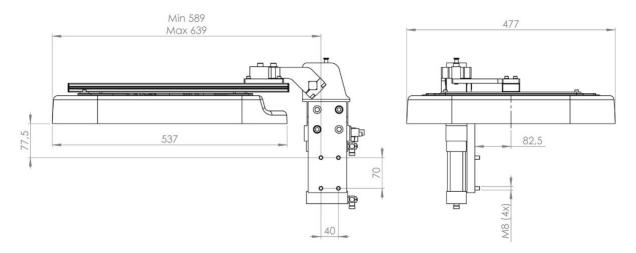
Dust cover with pneumatic tilting clamp large P8327 (drawing above) and P8377 should be used together with tool changers TC240, TC480, TC720 with corresponding tool attachments.
