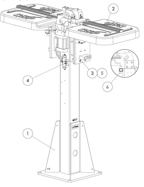
Tool parking system double P8366 and P8386 shall be used together with the tool changers TC240, TC480, TC720 and corresponding tool attachments. P8366 should be used together with safety signal modules P7501-xxx. P8386 can be used together with tool in stand sensors assembly, P8364, and tool present sensors, P8312.
