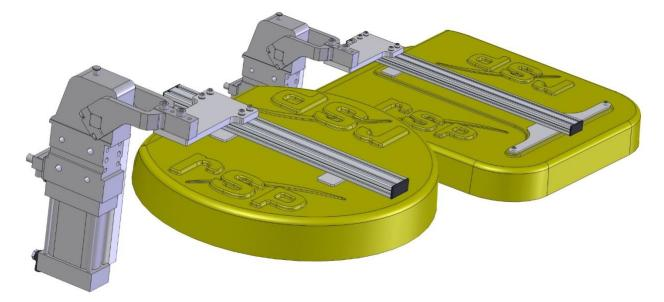
The options P8327, P8377 and P8379 (dust covers with pneumatic tilting clamp) shall be mounted on the tool stand column P8380. The dust covers are used for effectively protecting the tool and tool attachment when docked on the tool stand. The tilting angle is adjustable within the range of  $10^{\circ}$ – $135^{\circ}$ . The default tilting angle for tool parking system single is fully open, 135° and the default tilting angle for tool parking system double is 90°.
