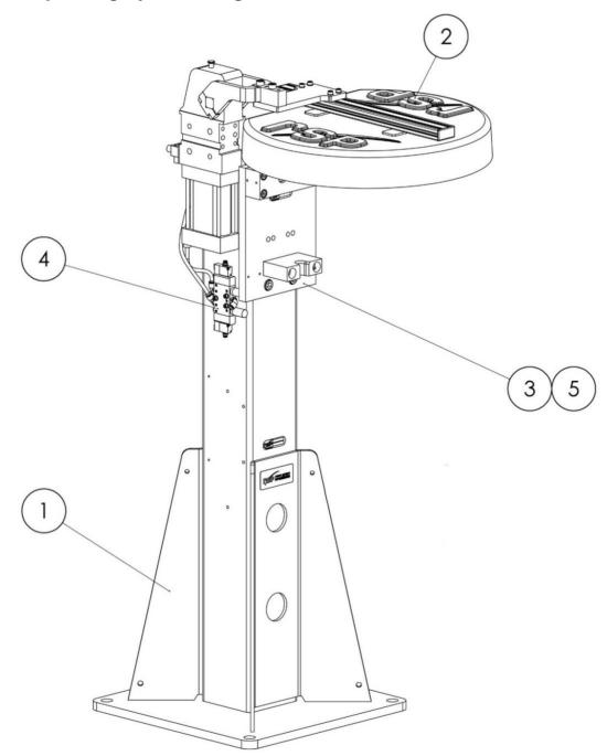
Tool parking system single P8383 shall be used together with the tool changer TC500 and tool attachment TA500. P8383 can be used together with tool in stand sensor assembly, P8364, and tool present sensor, P8312.
