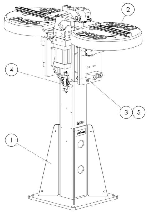
Tool parking system single P8384 shall be used together with the tool changers TC500 and tool attachments TA500. P8384 can be used together with tool in stand sensors assembly, P8364, and tool present sensors, P8312.
