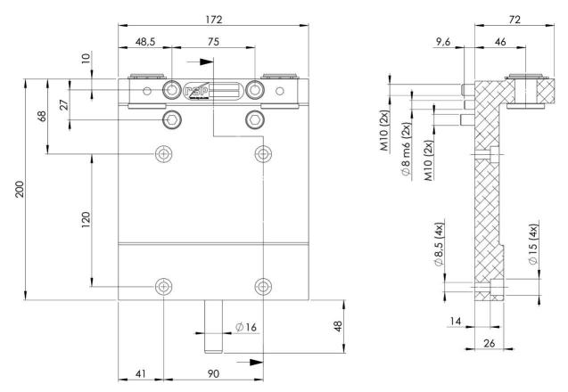
The tool plate P8303A, mounted on the tool attachment, gives together with tool hanger P8302 and tool stand column P8380 a robust tool parking system for easy tool changing.
