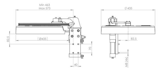
Dust cover with pneumatic tilting clamp small P8379 should be used together with tool changer TC500 with tool attachment TA500.
