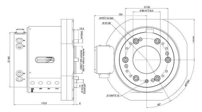
Swivel S250-8E transfers 8 pneumatic channels and 17 electrical signals to the tool.
