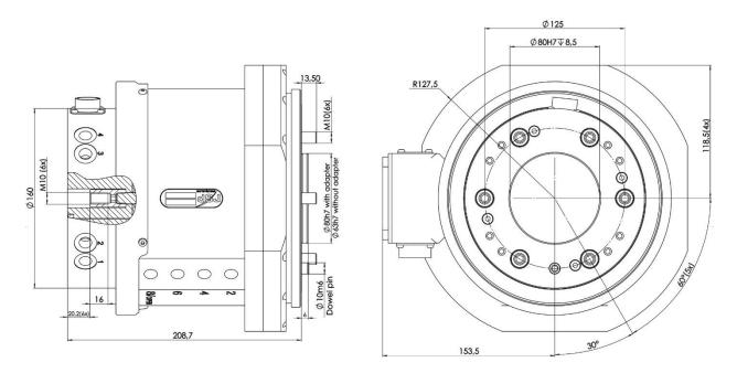
Swivel S250-8E Sealed transfers 8 pneumatic channels and 17 electrical signals to the tool.
