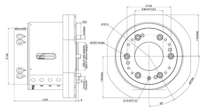
Swivel S250-8 transfers 8 pneumatic channels to the tool.
