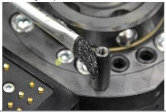
Apply a small amount of grease (Renolit HLT2) on the guide pins.
