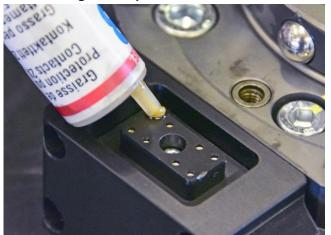
Apply a small amount of grease (Electrolube SGB) in each signal and servo power socket.
