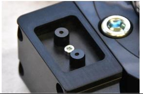
Check that the area around the high voltage socket is clean. For cleaning and lubrication see section 3.2.3.
