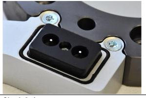
Check that the high voltage pins are clean. For cleaning and lubrication see section 3.2.4.
