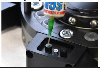
Apply a small amount of grease (Electrolube SGB) in the high voltage sockets.
