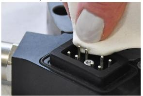
Wipe clean the signal and servo power pins with a cotton swab.
