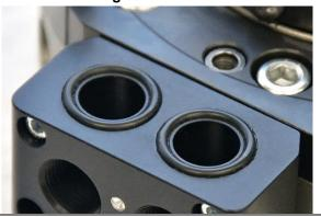
Check that the air sealings are clean. For cleaning see section 3.2.3.
