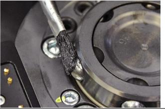
Apply a small amount of grease (Renolit HLT2) on the locking balls.
