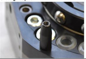
Check that the guide pins are greased. For cleaning and lubrication see section 3.2.3.
