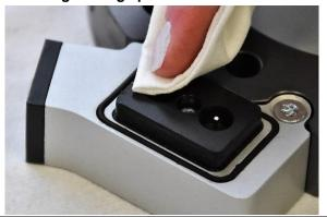
Wipe clean the high voltage pins with a cotton swab and the surface around the pins with a lint free cloth!
