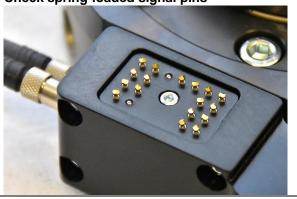
Check that the spring-loaded signal pins are clean. For cleaning see section 3.2.3.
