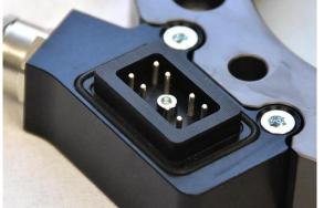
Check that the signal and servo power pins are clean. For cleaning and lubrication see section 3.2.4.
