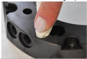
Wipe clean and apply small amount of grease (Renolit HLT2) inside the guide pin holes.
