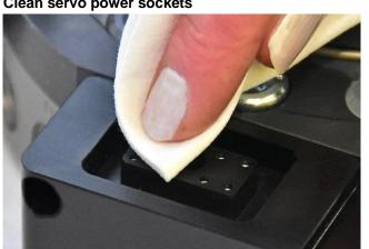
Wipe the areas around the signal and servo power sockets clean.
