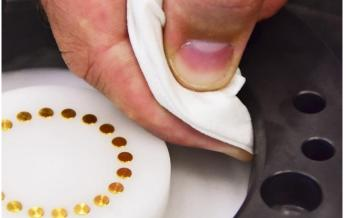
Clean the cavities of the locking balls with a lint free cloth.
