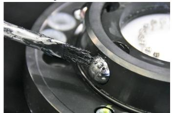
Apply a small amount of grease (Renolit HLT2) on the locking balls.
