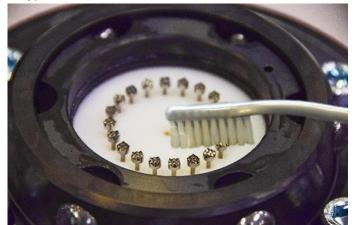
Clean the contact surfaces of the spring-loaded signal pins with a nylon brush.
