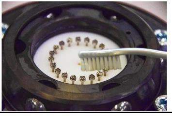
Clean the contact surfaces of the spring-loaded signal pins with a nylon brush.
