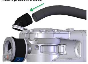
Mount the protective hose by pushing it distinctly into the elbow gland until locking.
