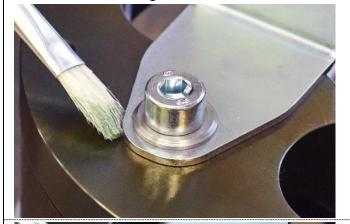
Apply a small amount of grease (Renolit HLT2) on the surfaces between the hose/cable guide and the CiRo-shaft and the hose/cable guide and the bushing, respectively.
