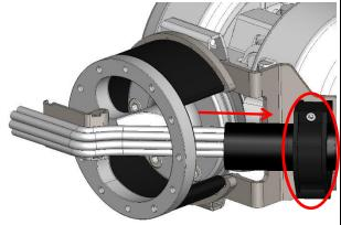
Loosen the screws holding the hose clamp and remove the protective hose, including cable and hoses, from the CiRo and hose clamp.
