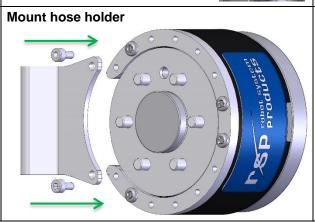
Mount hose holder on the backside of the CiRo housing, through the mounting ring.
