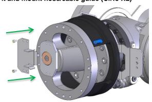
Fasten the hose/cable guide and bushing with the enclosed screw. Use a torque wrench for tightening (see tightening torques in section 1.3).
