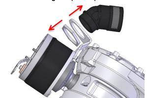
Unscrew the nut holding the cable gland and remove it.
