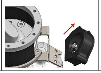
Unscrew the screws holding the hose clamp and remove it (when applicable).
