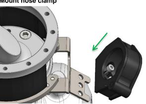
Mount a hose clamp with two screws on the hose holder. Use a torque wrench for tightening (see tightening torques in section 1.3).
